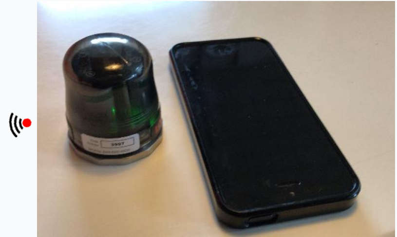
Ventus RCM wireless and battery powered sensor node located next to iPhone 5
